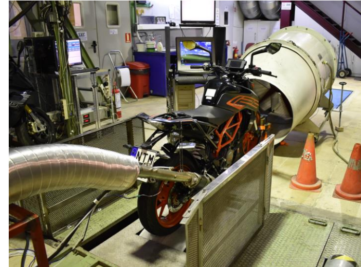
In-lab emissions testing by EMISIA in LAT
